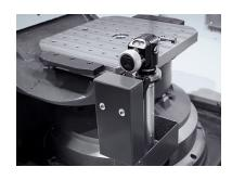
An automatic probe arm stores the tool setting probe in a protective compartment during machining operations. When the tool probe is needed, an M104 code activates the automatic probe arm to lift the probe and lock it into place. When probing is complete, an M105 retracts the probe to its protective compartment.
