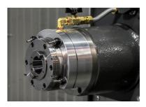
cylindrical design prevents chips from collecting on top.
