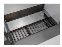
The EC-400/500 Series machines feature a wider belt-type chip conveyor positioned in the center of the machine, directly under the spindle, for vastly improved chip management. The steep walls of the interior enclosure easily funnel chips to the conveyor.
